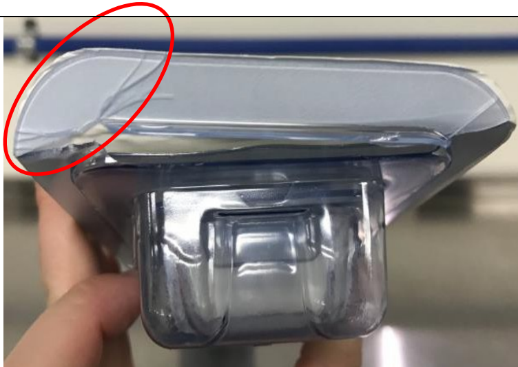
Fig 1. Outer Tray Flange Broken
