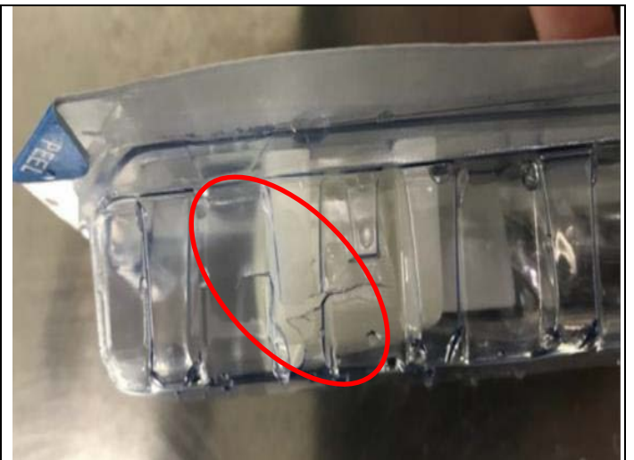
Fig 2. Inner Tray cracks near the plug
