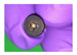
Zimmer Biomet is conducting a lot specific medical device field action for the Oxford Unicompartmental Knee Drill Guides (Phase 3/Domed Lateral) due to the incorrect raw material used by the supplier in the manufacturing of the screw component, which material could potentially lead to corrosion.
