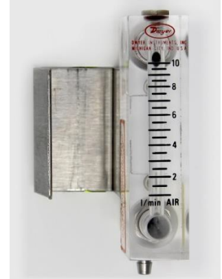
Backup external flowmeter, part number 147361. Use an external flowmeter to confirm true flow rate.
