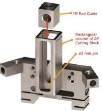
See pictures above. The rectangular column of the AP Cutting Block is a slot in which the IM Rod Guides are placed. This slot is open on the upper side and 'closed' by the  $\emptyset 2$  mm pin on the lower side. The only function of the  $\emptyset 2$  mm pin is to prevent the IM Rod Guide falling through the slot during assembly and disassembly, is has no function during the surgery itself due to the fact that the IM Rod Guide is positioned above the pin by the IM Rod during surgery.
