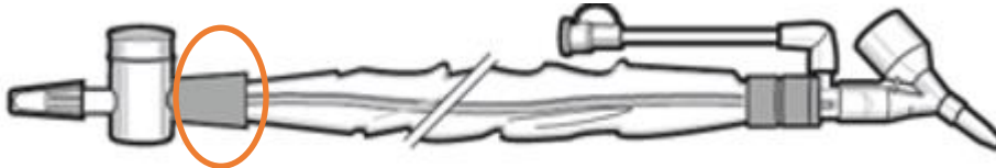
Figure 1: Location where the potential occlusion was identified. The blockage is not visible to the user.
