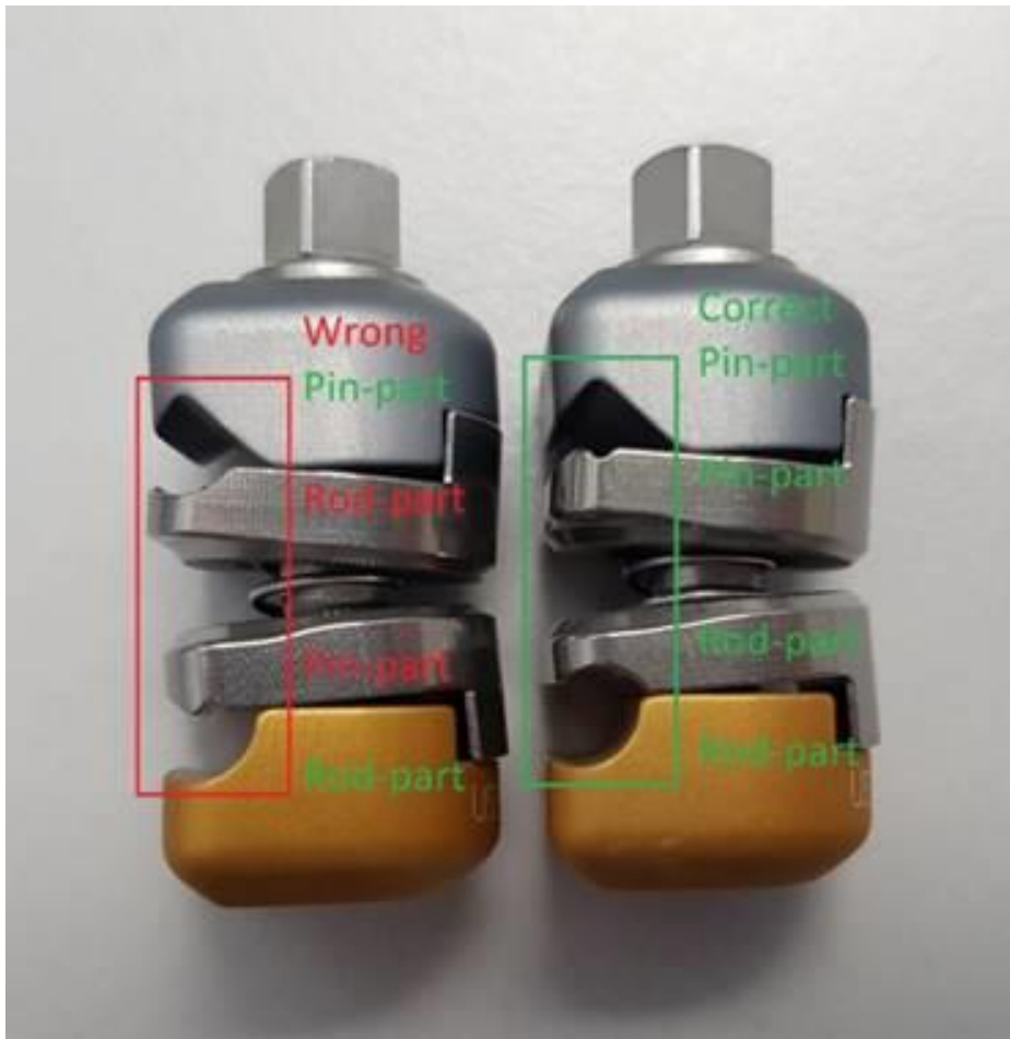
Figure 1. Left: wrongly assembled, Right: Coupling assembled correctly.
