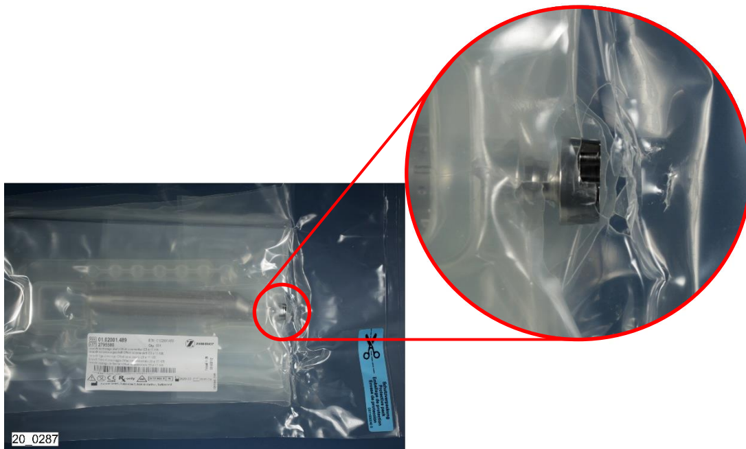
Picture 1: Damaged Packaging of Innex Anchorage Stem
