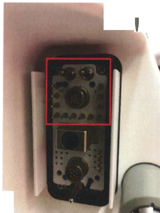
figure 2: example of XIO connector contact pin area which must not be touched
