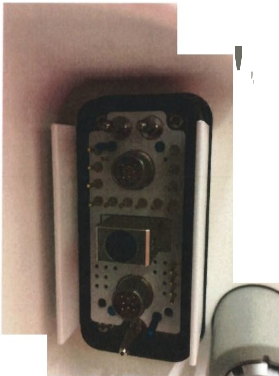
figure 3: example of XIO connector without the plug of the main cable being plugged in
