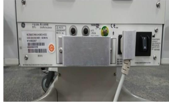
Figure 3: Servo Oxygen module is NOT installed
