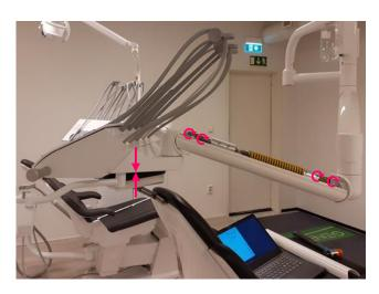
3. Remove the back axles. Save the axles and lock rings.
