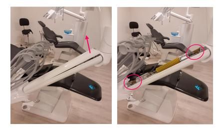
2. Position the bridge. Raise the bridge on the patient chair headrest. Raise the bridge until the axles are loose and removable.
