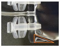
The MACS <u>logo should be completely visible</u> <u>and the seals</u> near the Twist-off-Ports should reach completely to the edge of the Freezing Bag. This is safe to use.
