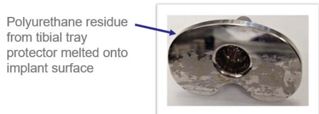
Image 2: Example of residual material on implant surface
