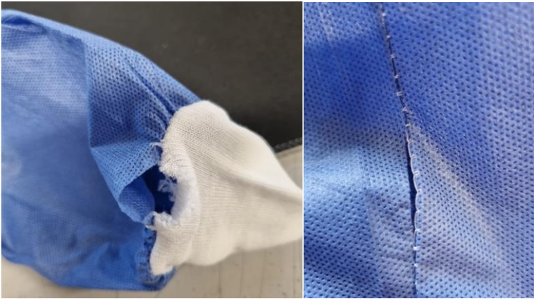
Figure 1: Sewing defect on cuff and seam
