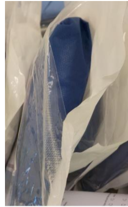
Figure 2: Open seal defect
