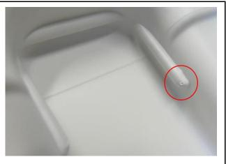
Example for a crack in intellipack packaging tray
