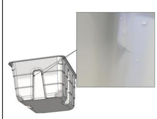
Area on the intellipack packaging tray where the failure was detected with example of crack
