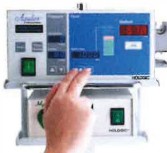
Figure 1 Note: To show the total inflow volume please hold down both the Increase- and Decrease-deficit limit -buttons.
