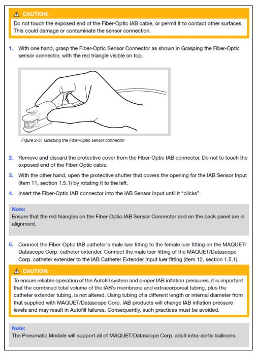
In step 4, when the Fiber-Optic connector is inserted into the IAB Sensor input until an audible "click" is confirmed, ensure that you are not using excessive force as that can lead to damage to the Cardiosave.
