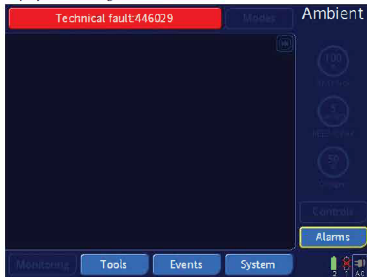
Figure 1: The display indicates “Ambient State”, and a red message with a Technical Fault number (example, a different Technical Fault number might be displayed)
