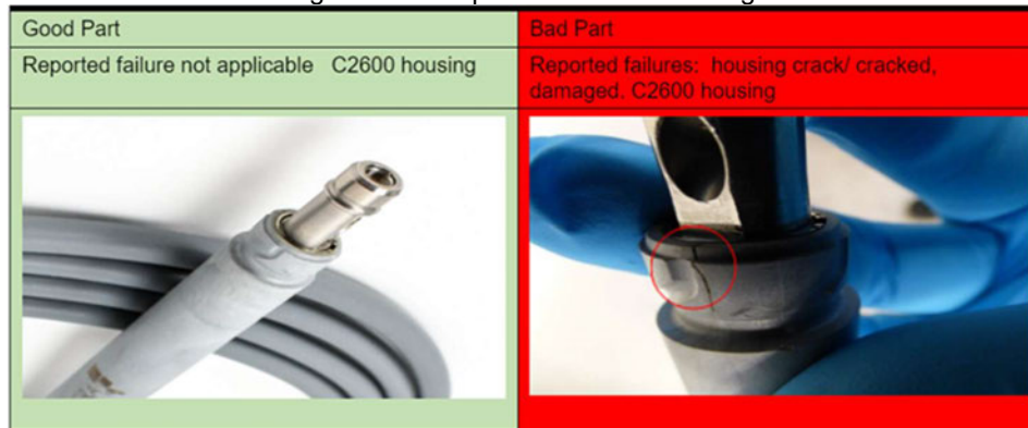
Figure 1: Example of Cracked Housing
