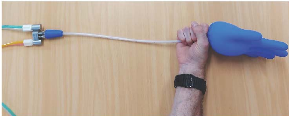
Figure 6: Pressure test. Ventilation is running. Glove inflates.
