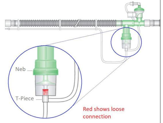
Figure 1: IPPB Breathing system schematic showing zoom detail of nebuliser and supply line T-Piece connection
