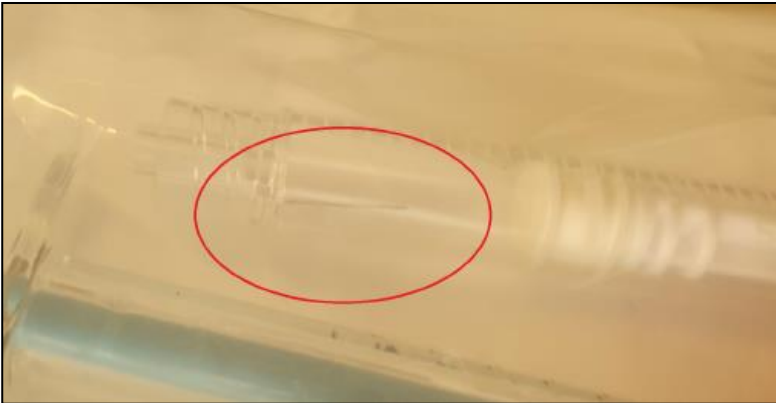
Picture 1: crack on syringe body
